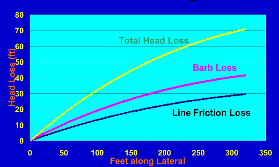
Friction Loss Along Lateral (2 ft/s flushing)
