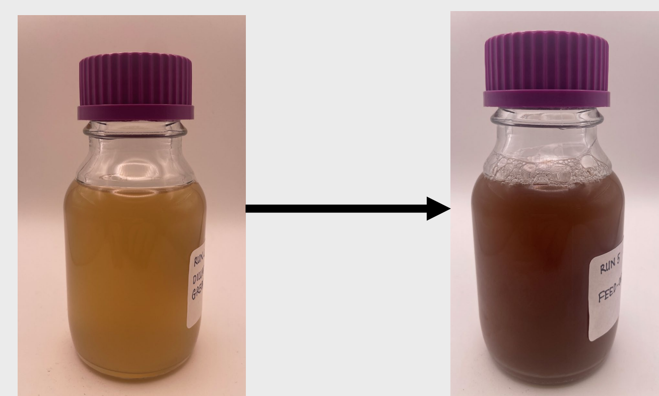
Liquid digestate (6 liters → 1 liters of concentrate)
